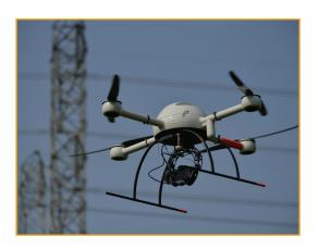
Con Edison is deploying unmanned aircraft systems (UAS), commonly called drones, to inspect transmission lines and to make sure trees and vegetation do not have the potential to make contact. The drone inspections are faster than traditional inspections and enhance worker safety.
